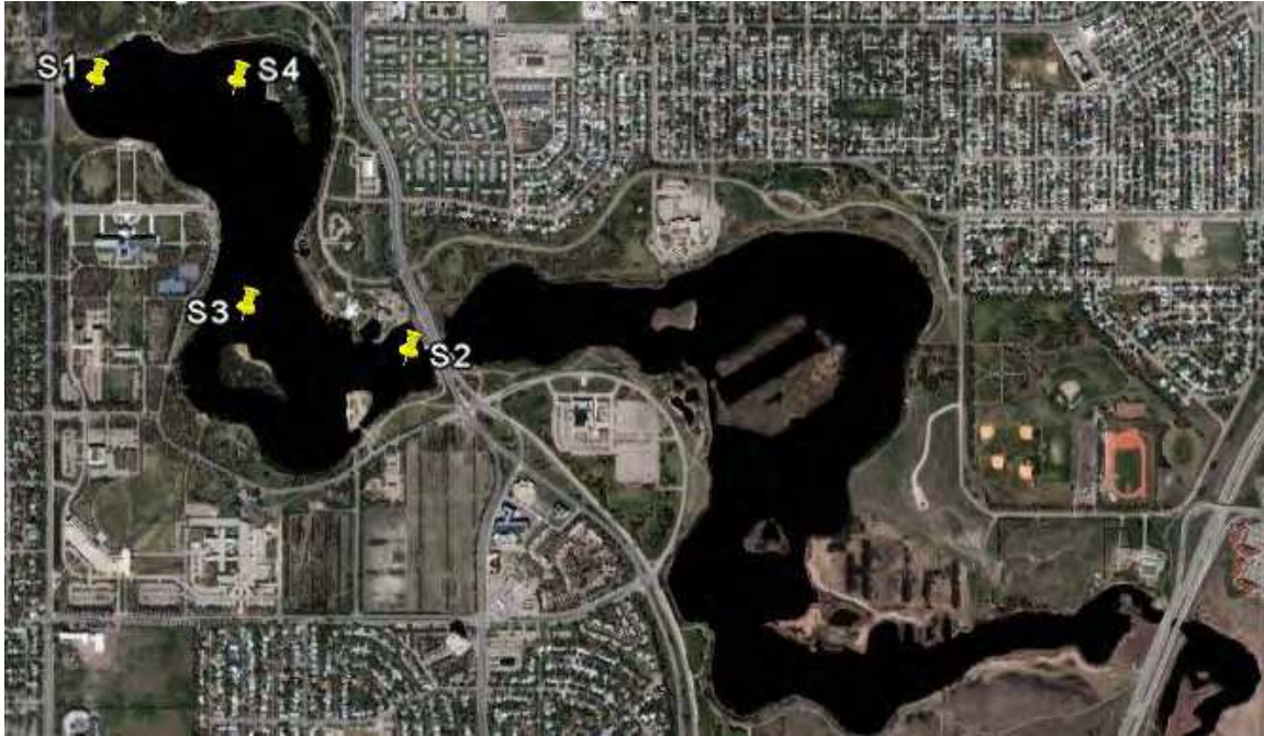
Figure 1: Wascana Lake Sampling locations. Water flows in at S2 (Broad St.) and exits at S1 (Albert St.).
