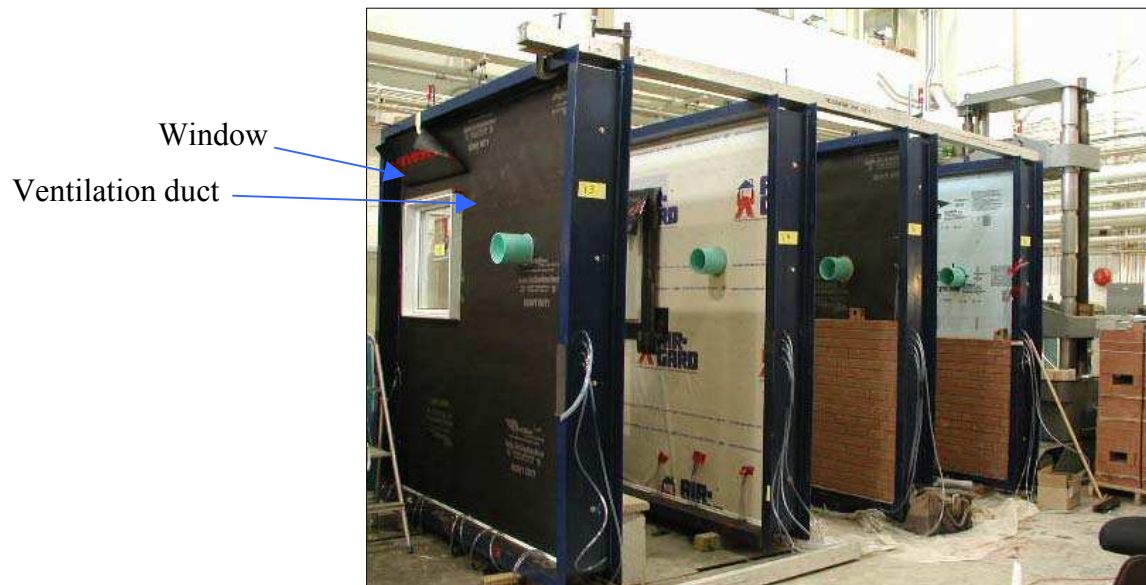
Figure 1. Full-scale 2400-mm by 2400-mm test specimens shown at different stages of fabrication. Four of the 17 wall specimens included brick veneer.
