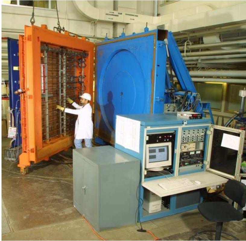
Figure 2. IRC researchers use the Dynamic Wind and Wall Testing Facility to expose wall specimens to wind-driven rain loads and investigate where water (and how much) gets deposited into the layers of the wall assembly. The facility comprises a water spray system that simulates the action of rain; a blower to simulate wind effects; and a piston that, through its cyclic action, varies air pressure to simulate wind gusts.
