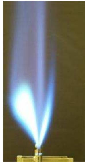
Figure 3. Direct visualization of a stratified V flame stabilized in the gradient of a partially premixed isooctane-air mixture
