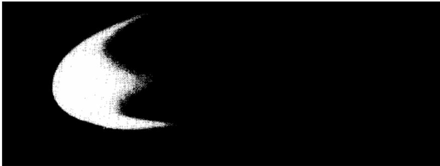
**Figure 1. Triple flame observed in a horizontal methane/air mixing layer [7]**
