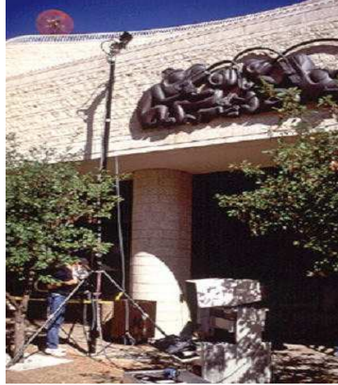
Figure 1: Range sensor mounted on a tripod; stability is paramount in acquiring high accuracy range images. Accuracy of range data is the combination of the range sensor and its mechanical supporting structure. Vibrations and oscillations induced by winds or passing vehicles can seriously affect accuracy.
