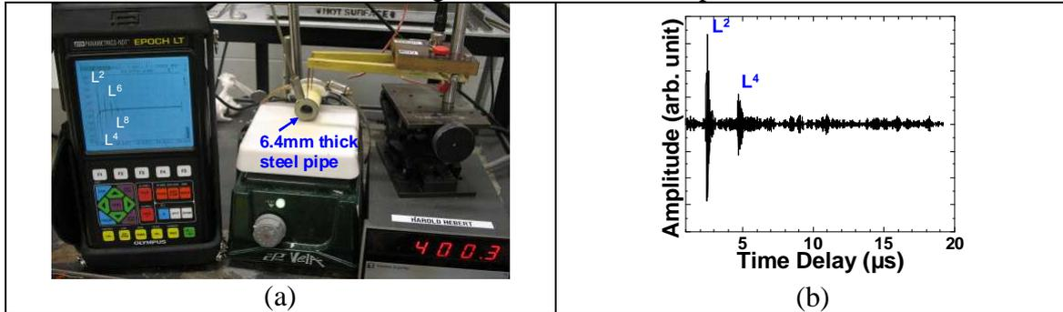
Figure 2. (a) Measurement setup and sample for an IUT made of BIT/PZT composite film at 150°C using an EPOCH LT and performed in pulse-echo mode; (b) Measured ultrasonic signals using laser generated ultrasound and IUT as the receiver in pitch-catch mode at 400°C.
