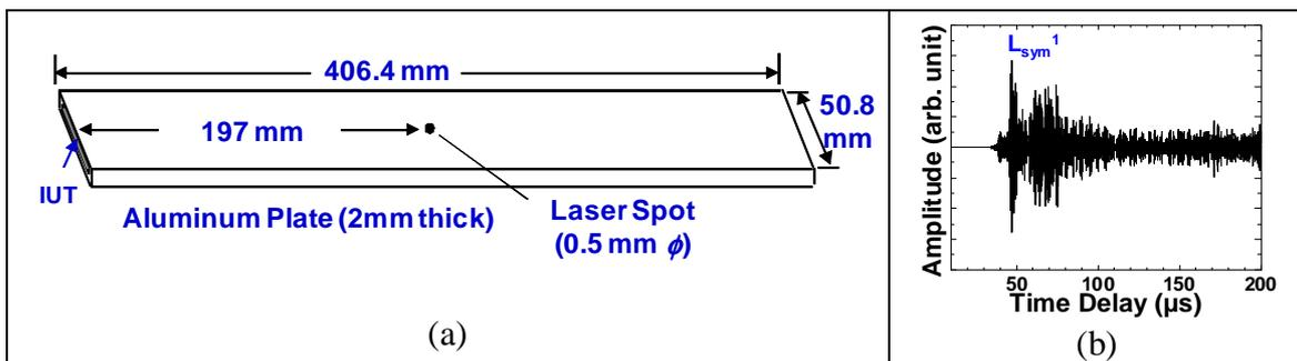
Figure 4. (a) Sample and measurement arrangement for symmetrical PAWs; (b) Measured ultrasonic signals at room temperature.
