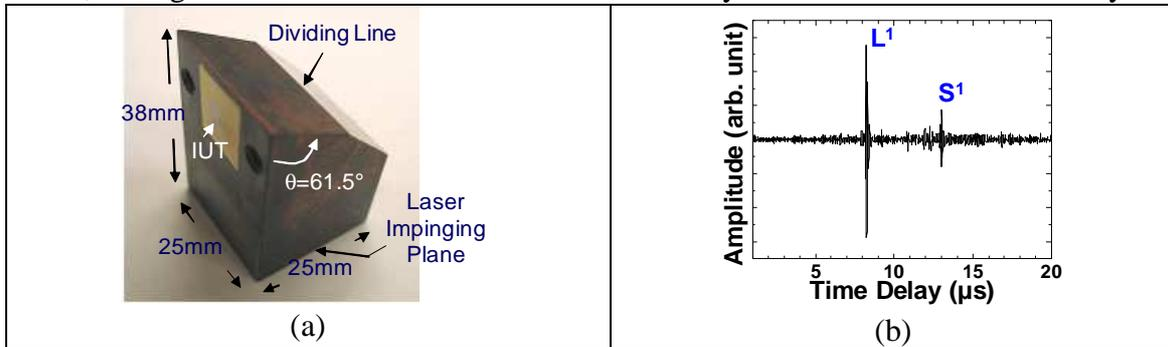
Figure 3. (a) Sample and measurement arrangement for both L and S waves; (b) Measured ultrasonic signals using laser generated ultrasound and IUT shown in Figure 3a as the receiver at  $400^\circ\text{C}$ .
