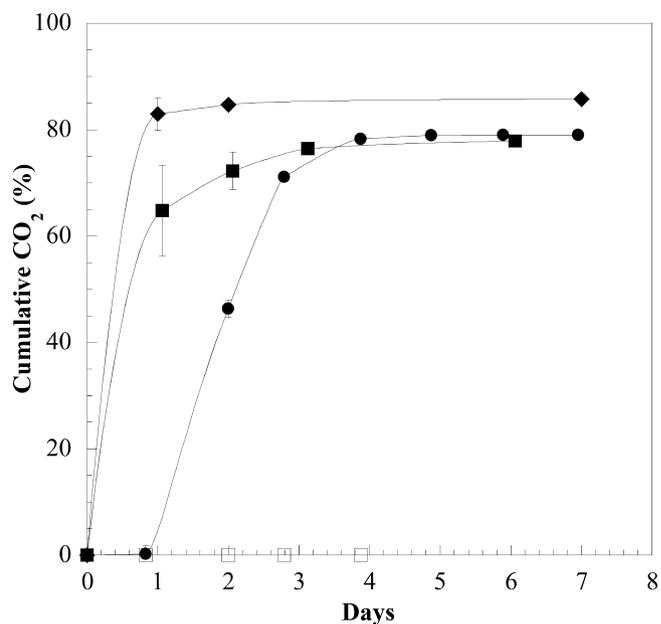
FIG. 1. Mineralization of [<sup>14</sup>C]NDMA into <sup>14</sup>CO<sub>2</sub> by washed cells of *R. ruber* ENV425 initially cultivated in TSB (●), BSM with glucose (■), or BSM with glucose and NDMA (◆). Values from samples with TSB only (no cells) are also shown (□). Values represent means and standard deviations of the results obtained using triplicate samples.
