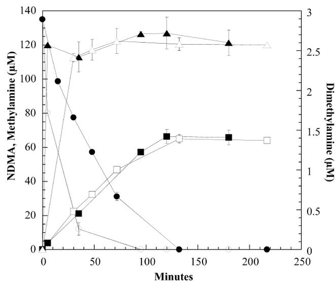
FIG. 4. Liberation of MA and DMA from NDMA by *R. ruber* ENV425 after growth on glucose and NDMA (closed symbols) or propane (open symbols). Symbols: NDMA (●, ○); MA (■, □); DMA (▲, △).
