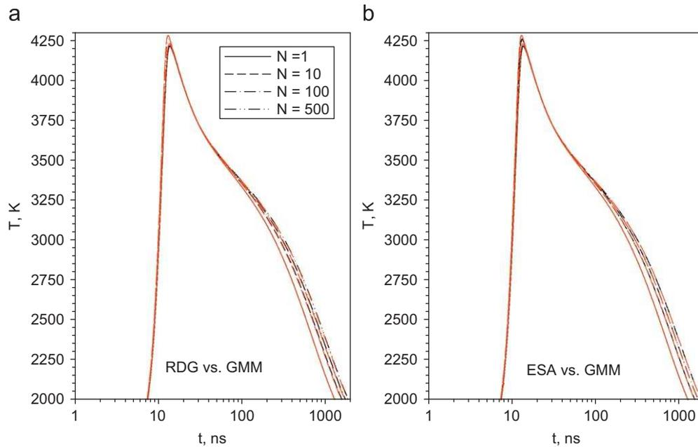
**Fig. 3.** Soot temperature histories predicted by three aggregate absorption submodels for  $F_0 = 1.5 \text{ mJ/mm}^2$ . See Fig. 2 for legends. (For interpretation of the references to colour in this figure legend, the reader is referred to the web version of this article.)
