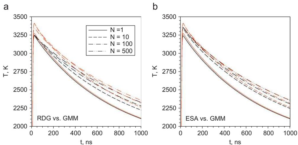
Fig. 2. Soot temperature histories predicted by three aggregate absorption submodels for  $F_0 = 0.65 \text{ mJ/mm}^2$ . Black lines are either RDG (a) or ESA (b). Red lines are GMM. (For interpretation of the references to colour in this figure legend, the reader is referred to the web version of this article.)
