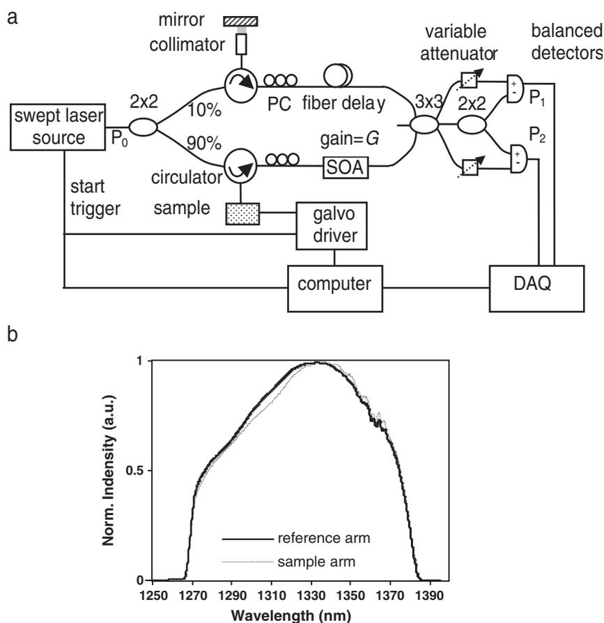
Fig. 1. (a) Experimental setup of our QSS-OCT system with a balanced  $3 \times 3$  and  $2 \times 2$  quadrature MZI and an SOA for the amplification of the signal back-scattered from the sample. (b) Measured normalized spectra of light source reflected from reference arm (solid line) and amplified sample arm (dot line).
