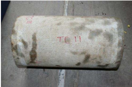
(a) 300 mm sub-sample for crush test
